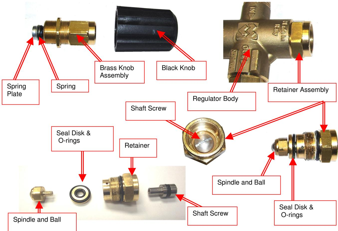
9. Use a synthetic grease with Teflon such as Ultra-Slick or Super-Lube to lubricate the seals on the shaft screw and seal disk.
