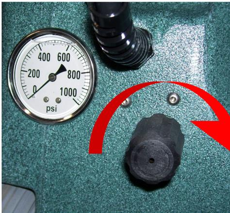
To increase the solution pressure, turn the regulator knob clockwise.
